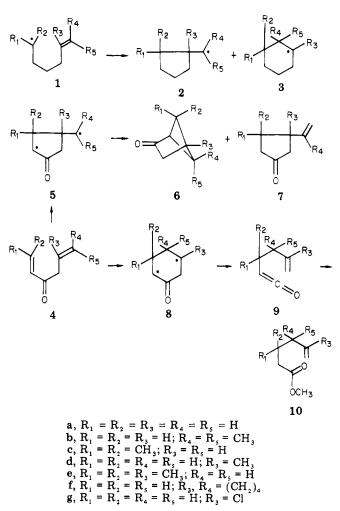
4c in refluxing *p*-xylene and obtained nearly a quantitative yield of 6c,<sup>12,13</sup> the desired product.
